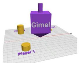
**Description:** Students will create a dreidel in BlocksCAD by orienting and engraving text onto the four sides of a dreidel using the **rotate**, **translate**, and **difference** blocks. Students will play a BlocksCAD version of the game dreidel.
